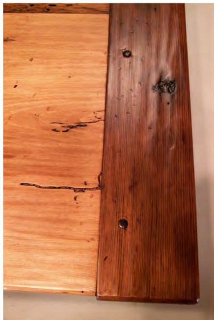
DETAIL OF TOP Pinned breadboard end
