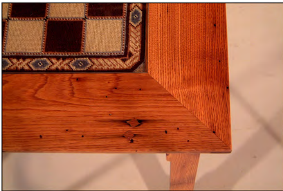
DETAIL Spline mitered corners
