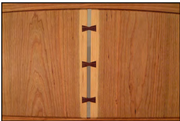
DETAIL OF HEADBOARD Gap in panel, "sutured" together w/ walnut butterfly keys
